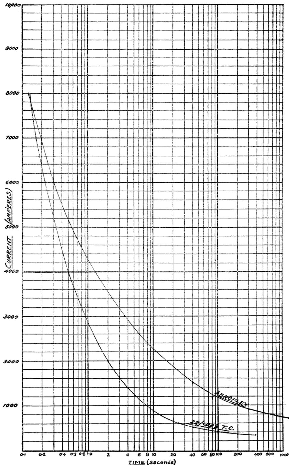
FIG. III.—TIME-CURRENT CURVES FOR AEROFLEX FUSES (500 AMP RATING) LOCATED IN M.E.D. SUBSTATION, LICHFIELD STREET, AND HEAVIEST FUSE (22/029 T.C.) USED IN SERVICES FUSES AT MESSRS. J. BALLANTYNE AND CO. AT TIME OF FIRE
