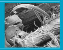
A scanning electron micrograph image of a fracture surface of a harakeke-epoxy composite. The finest filaments are individual macrofibrils torn from the fibres, and suggesting resin penetration into cell walls has occurred.
