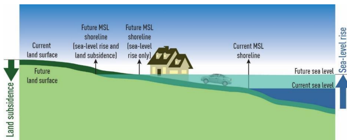
Figure 8-20: The difference in mean sea level (MSL) shoreline between absolute SLR (SLR only) and relative (local) SLR where land subsidence occurs (SLR + land level changes).
