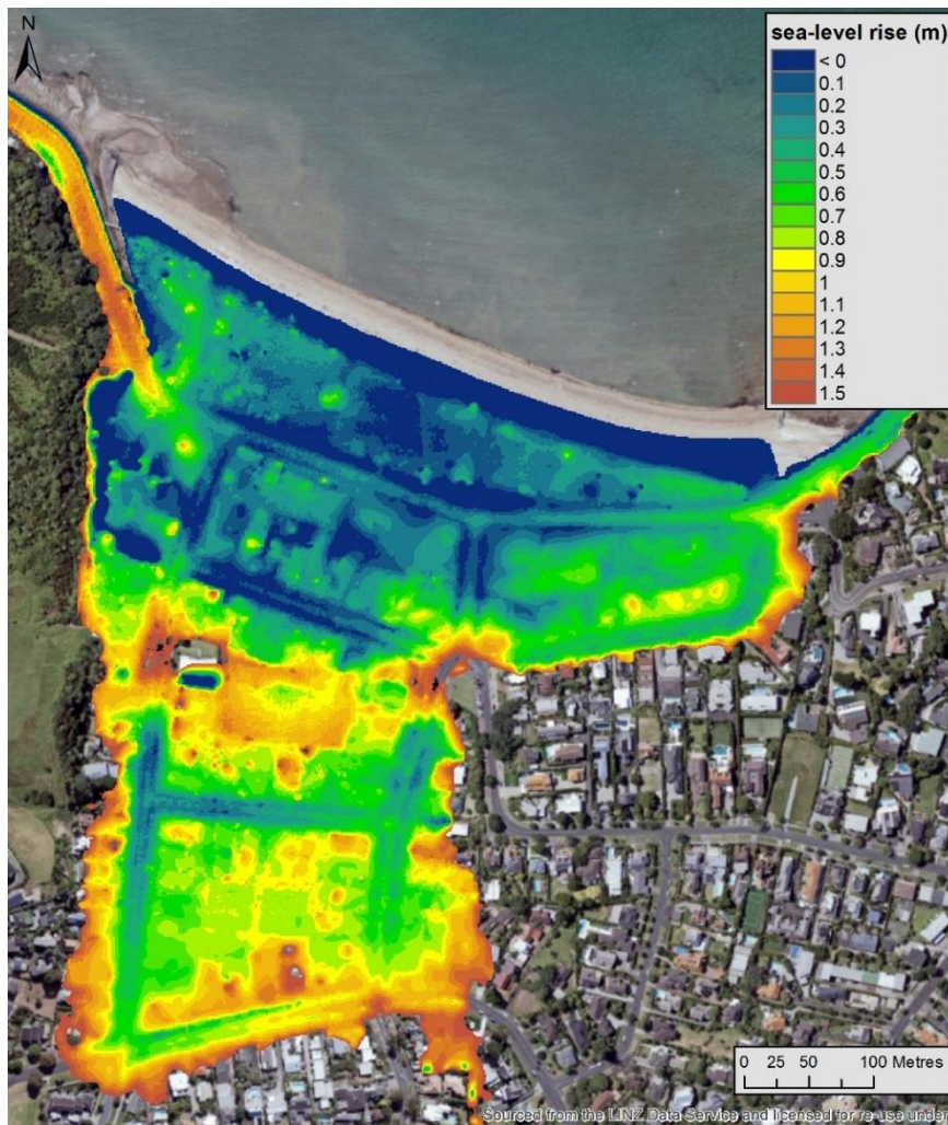
Figure 8-34: Effect of 0.1 m RSLR increments on coastal storm inundation exposure (1% AEP) at Mission Bay, Auckland. SLR increments have been added onto the 1% AEP storm-tide elevation, which was calculated for the present-day mean sea level Graphics: Sanjay Wadhwa, NIWA; based on Auckland Council LiDAR data. From Stephens et al. (2017).
