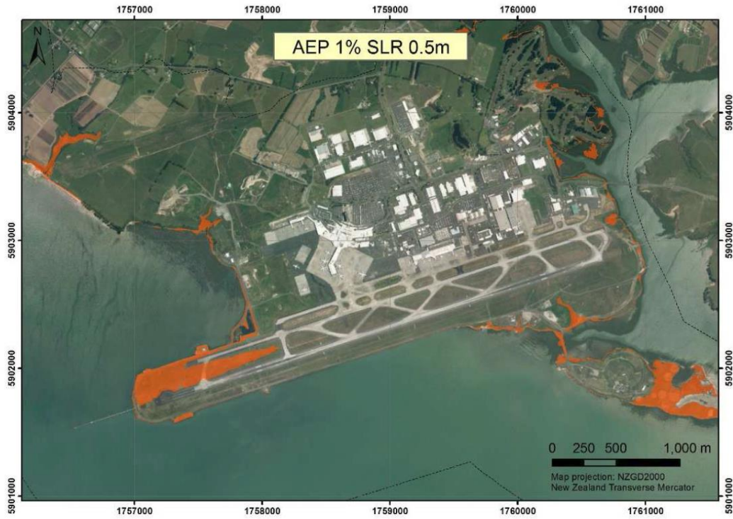
Figure 8-38: Map of the areal extent of coastal-storm inundation from a 1% AEP storm-tide + wave setup at present-day MSL + 0.5 m SLR at Auckland Airport. Orange shading = wet areas.
