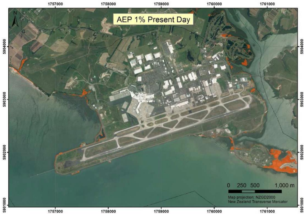
Figure 8-37: Map of the areal extent of coastal-storm inundation from a 1% AEP storm-tide + wave setup at present-day MSL at Auckland Airport. Orange shading indicates wet areas.
