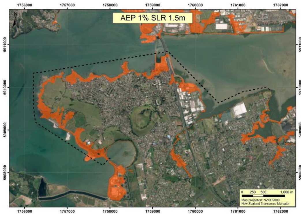
Figure 8-49: Map of the areal extent of coastal-storm inundation at Mangere from a 1% AEP storm-tide at present-day MSL + 1.5 m SLR. Orange shading indicates wet areas.
