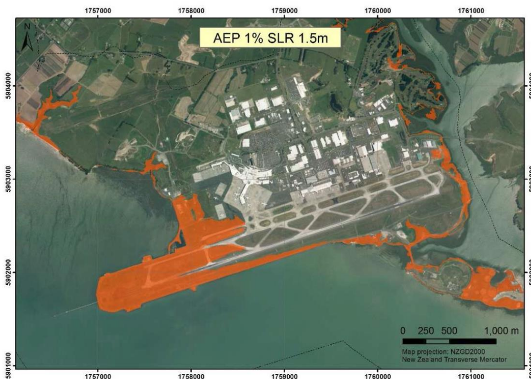
Figure 8-40: Map of the areal extent of coastal-storm inundation from a 1% AEP storm tide + wave setup at present-day MSL + 1.5 m SLR at Auckland Airport. Orange shading indicates wet areas.
