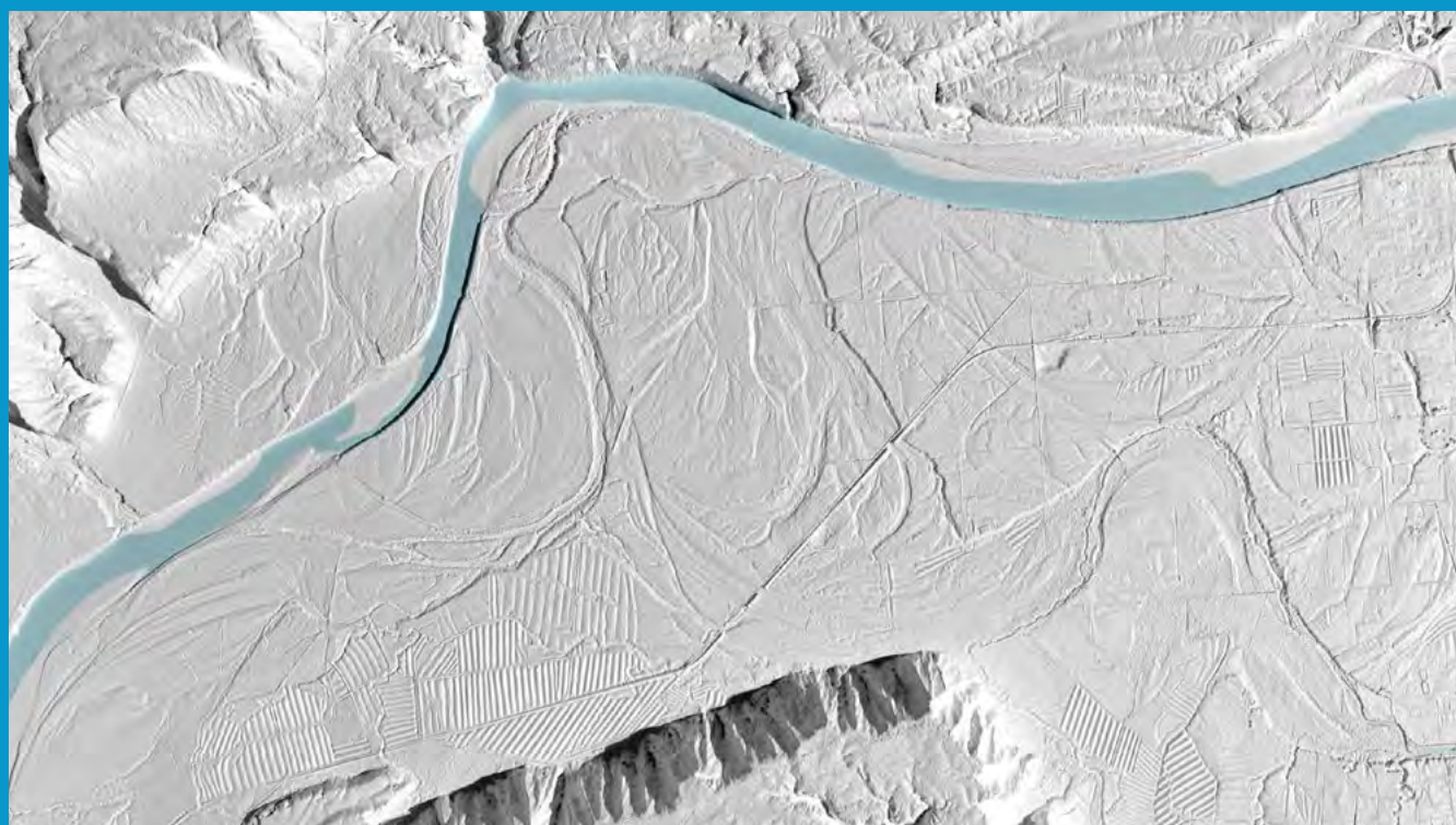
A digital elevation model snapshot of the Buller River and its floodplain, south of Westport. LiDAR captures information not easily seen in aerial imagery alone, such as pathways, rivers and streams.
