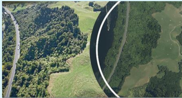
Because oblique imagery is captured at an angle, it provides more detail than a standard aerial photograph
