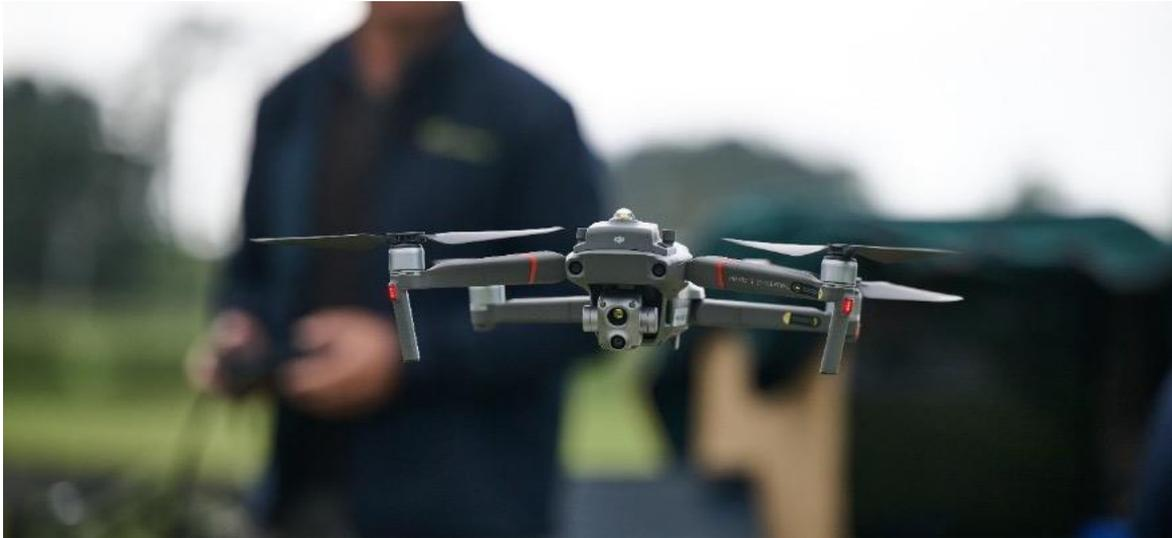
Drone being piloted with a hand-held controller. The drone carries thermal and visual light cameras, weighs around 900g, and can reach 72km/h. Credit: Craig McKenzie.
