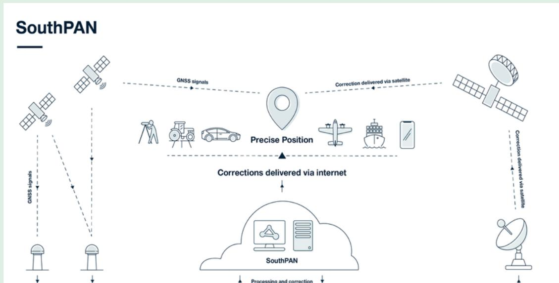
SouthPAN satellite-based augmentation system. Source: <https://www.linz.govt.nz/products-services/geodetic/southpan>
