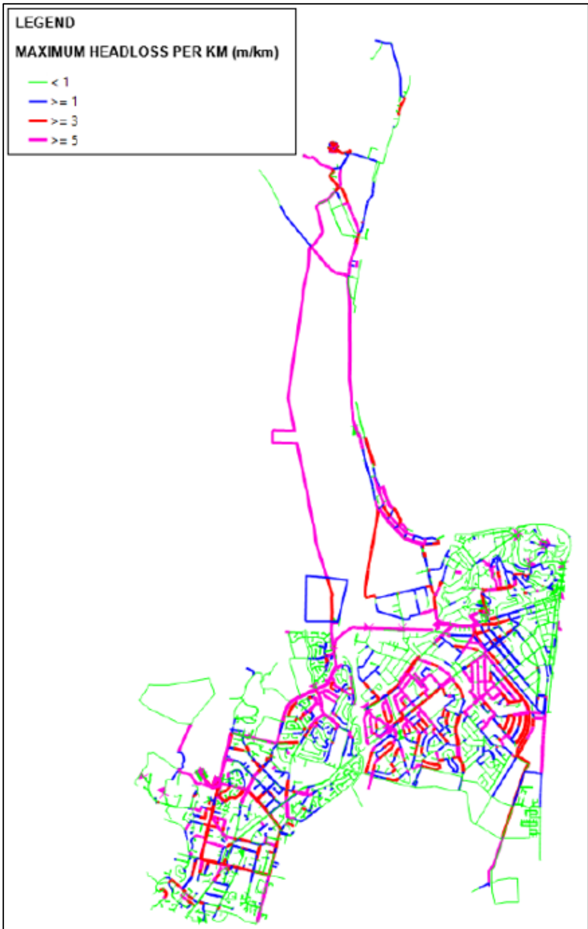
Figure 8 Maximum headloss per kilometre (m/km) for future model with updated growth data
