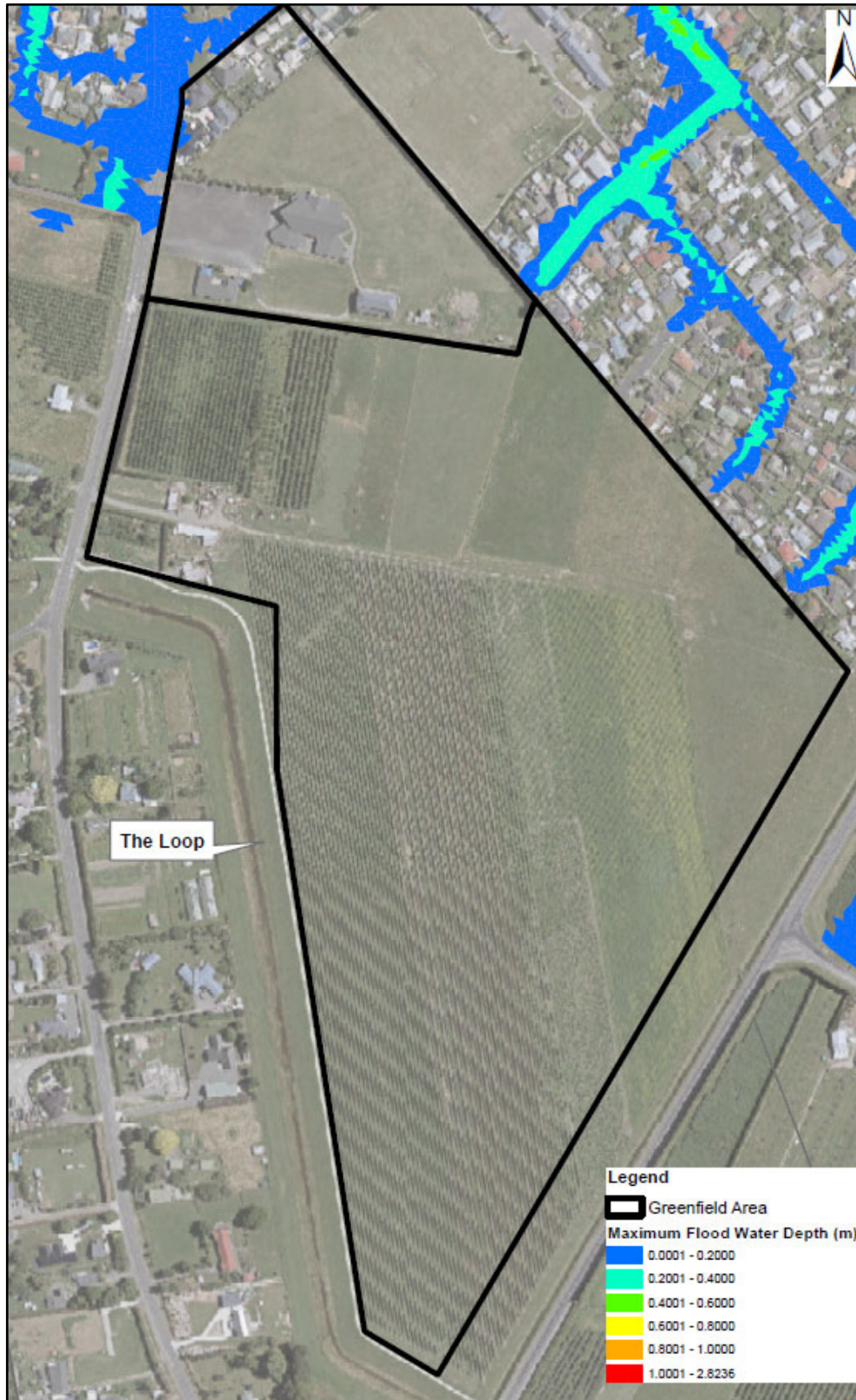
Figure 27 100 Year Flooding Extent – The Loop Site
