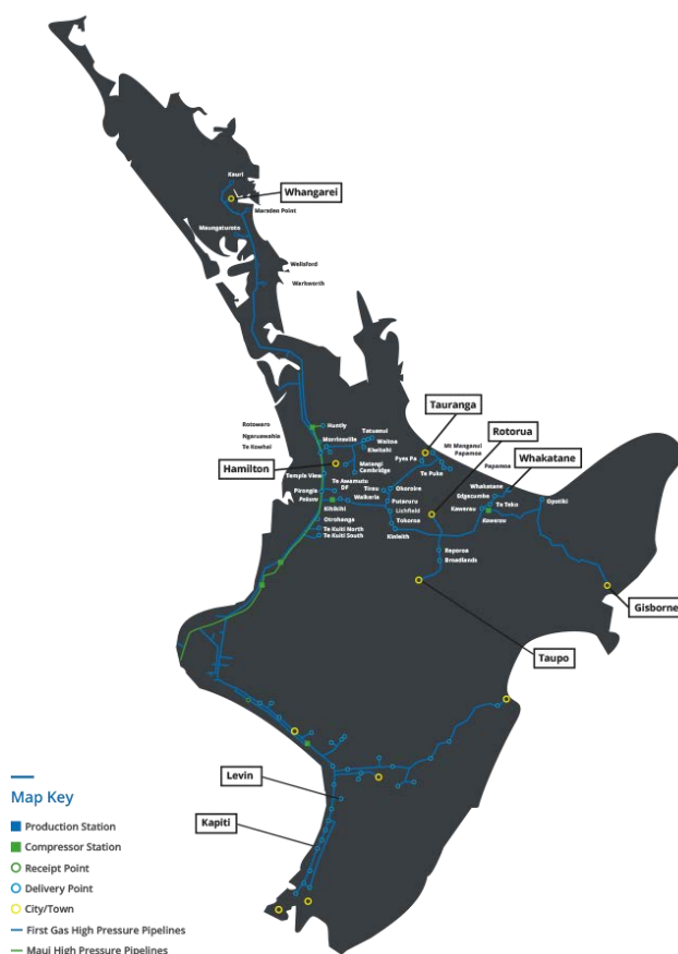
Figure 2.1: New Zealand natural gas transmission network
