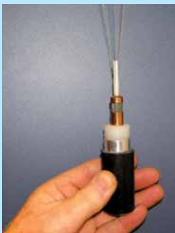
Deep-ocean fibre-optic cable with (outside to in) its black/white polyethylene sheaths, copper conductor, steel strength member and glass fibres.
