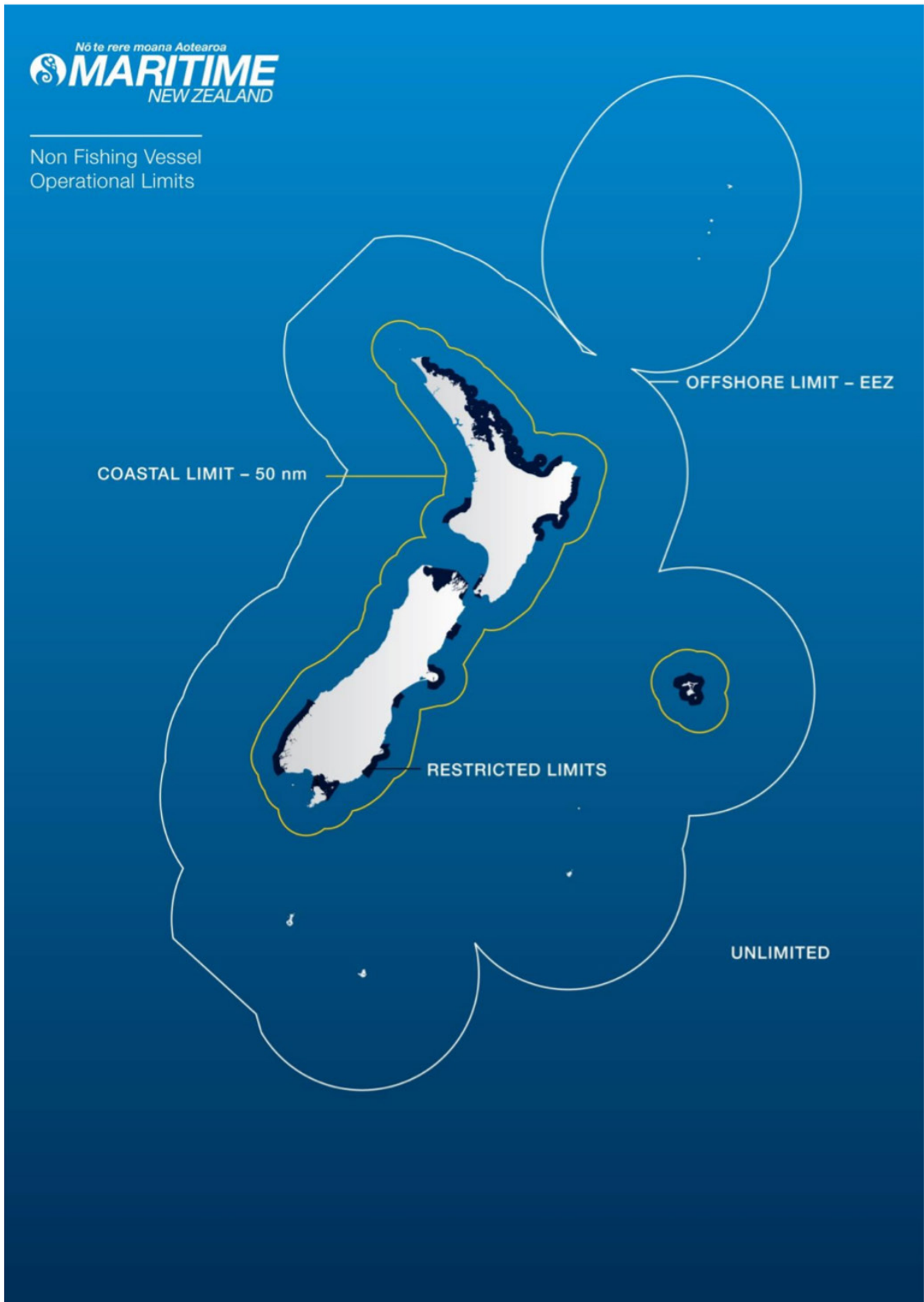
Figure 3: Maritime New Zealand operational limits diagram (non-fishing vessel operational limits) 28
