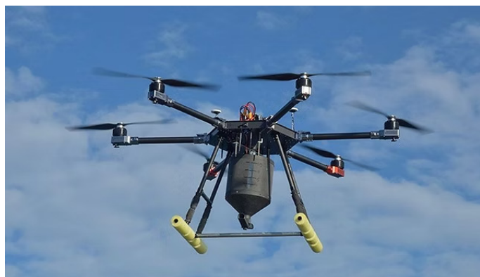
Figure 2: Seed pod drone system in development for cost efficient and fast native reforestation, Evinco (New Zealand). 4
